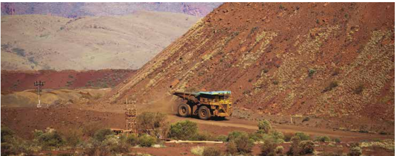
Iron ore mining requires the creation of huge waste dumps (as shown here) and the disposal of large volumes of water when mining drops below the watertable. Image: Krystle Wright
